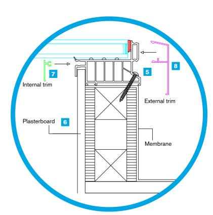
Lift the glazed rooflight onto the top of the kerb, keeping an equal spacing around the perimeter.
