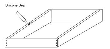
Once in place, screw through the rooflight outer frame into the kerb at 250mm centres. Make sure fixings are all secure.
